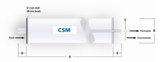
1. Each membrane element supplied with one brine seal, one interconnector (coupler) and four o-rings. 2. All RE4040 elements fit nominal 4.0 inch (102 mm) I.D. pressure vessels.
