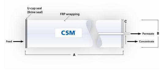
Each membrane element supplied with one brine seal, one interconnector (coupler) and four o-rings.
