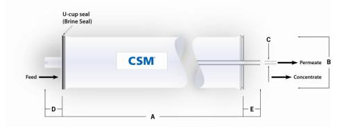
1. Each membrane element supplied with one brine seal, one interconnector (coupler) and four o-rings. 2. All NE2540 elements fit nominal 2.5 inch (64 mm) I.D. pressure vessels.
