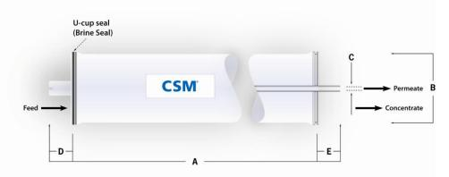
1. Each membrane element supplied with one brine seal, one interconnector (coupler) and four o-rings. 2. All NE4040 elements fit nominal 4.0 inch (102 mm) I.D. pressure vessels.
