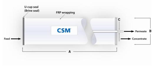
1. Each membrane element supplied with one brine seal, one interconnector (coupler) and four o-rings. 2. All RE8040 elements fit nominal 8.0 inch (201 mm) I.D. pressure vessels.
