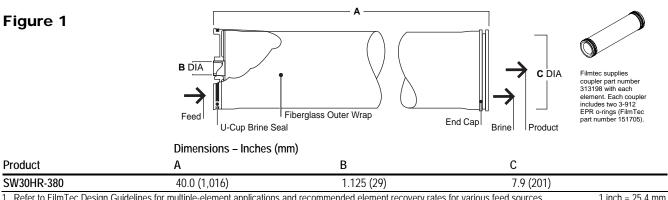
1. Refer to FilmTec Design Guidelines for multiple-element applications and recommended element recovery rates for various feed sources. 1 inch = 25.4 mm 2. SW30HR-380 fits nominal 8.00-inch (203 mm) I.D. pressure vessel.
