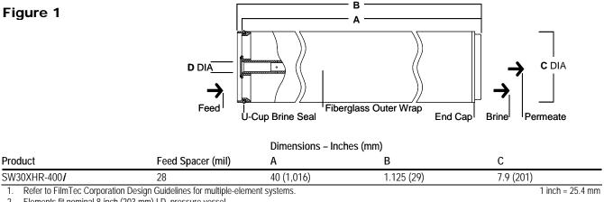
Elements fit nominal 8-inch (203 mm) I.D. pressure vessel. 2.
