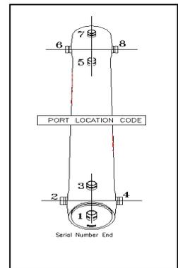
CODELINE BODY LABELS ARE PLACED AT 90° TO SERIAL NUMBER END AND AT 270° ON THE OPPOSITE SIDE END
